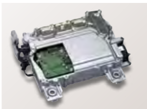
4WD rear inverter mounted in the new Prius
