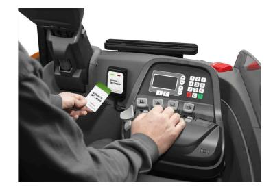
With smart access, drivers get a smart card to access the machines increasing security.
