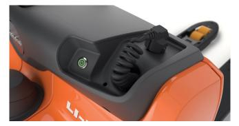
LWI160 - flexible energy solutions: three battery capacities, external or inbuilt charging, onbard lorry charging, wide range of chargers.
